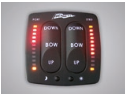
Trim tabs' adjustment panel, with indicators
