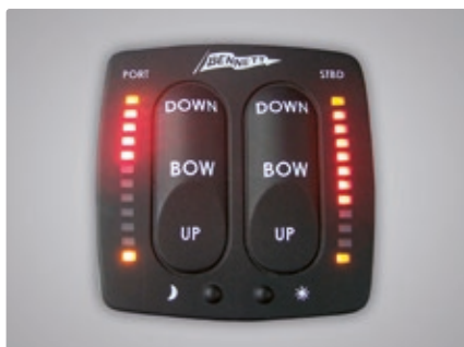
Trim tabs' adjustment panel, with indicators
